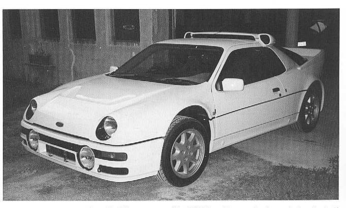
One of the design parameters of the RS200 Group B car was that the standard version should be a credible road car with a properly trimmed cockpit with even provision for a radio. Of all Group B rally cars, the RS200 is the most practical and comfortable car for everyday use.
